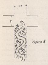
curves is recommended as greatly improving the appearance. There are no limiting conditions that demand a perfectly straight grade line from one intersection to another, either for sewerage, drainage or traffic. But it is very seldom that curves are found in use, though in residence districts they can be utilized to great advantage to the property. Very full data of the work on curves should be given and re-
