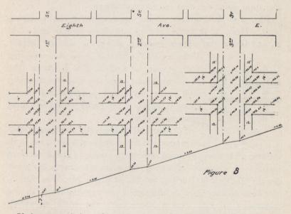
If the summit is to be on a curve the elevation of the curve should be worked out and given on the profile at least every twenty-five feet or oftener if the curve is sharp.
