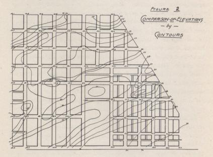
figures on the map giving the elevations, but if the map is contoured it is safer, and in most cases will so facilitate reaching the final conclusions as to more than pay for the extra labor. Fig. 2 illustrates how contours show the character of the ground.
