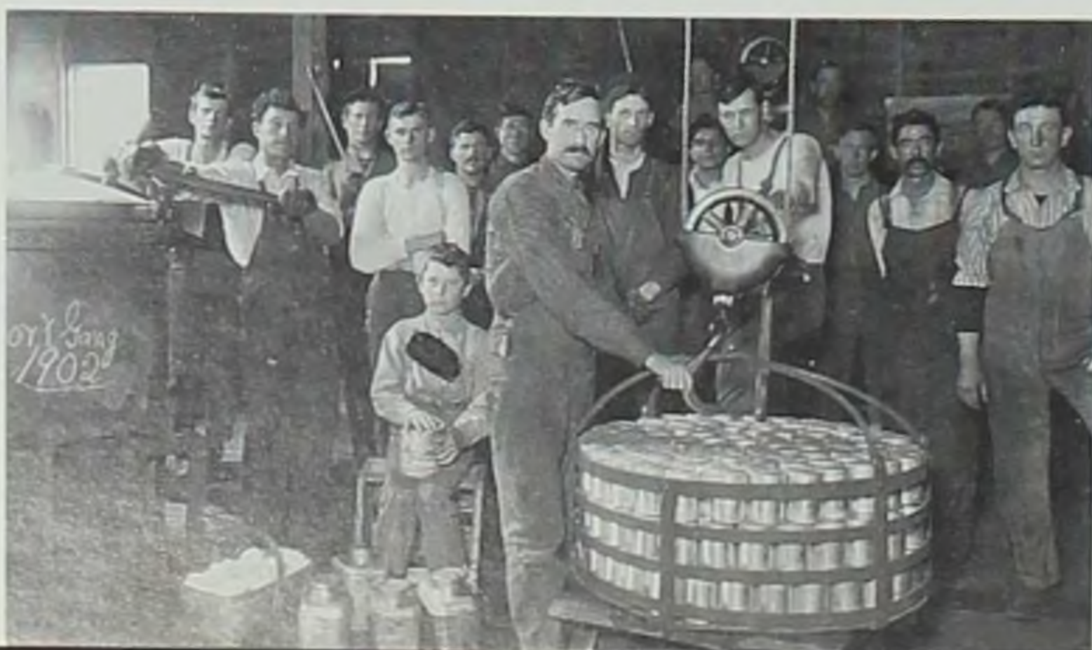
Left: Cans filled with produce are placed in enormous crate-like trays and then lowered into the retorts (above) for steam heating.
