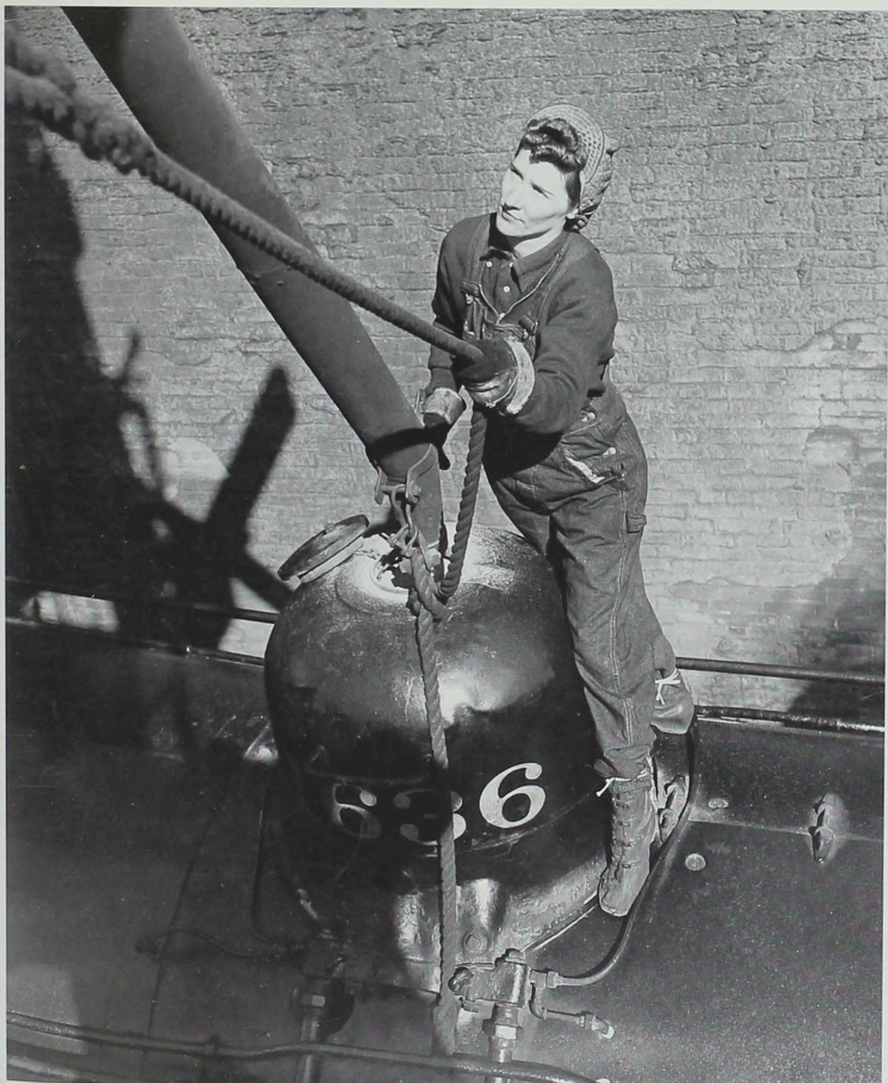
Edith Bennis, a former beauty operator, stands on top of a locomotive to service the sand dome. A year later, in anticipation of the end of the war, newspaper articles would focus on the problems of juvenile delinquency supposedly caused by women abandoning their children in order to work, and the need to find jobs for GIs who, it was assumed, would be coming home soon.
