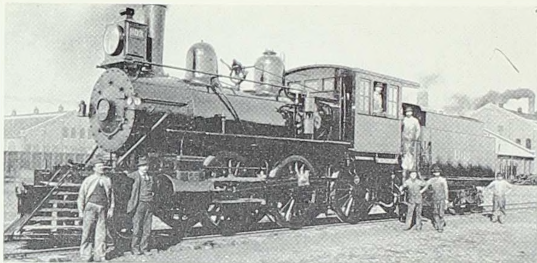
Mogul, or 2-6-0 type, locomotive at West Burlington shops in 1913. It was built by Rogers in 1892 and retired in 1927.
