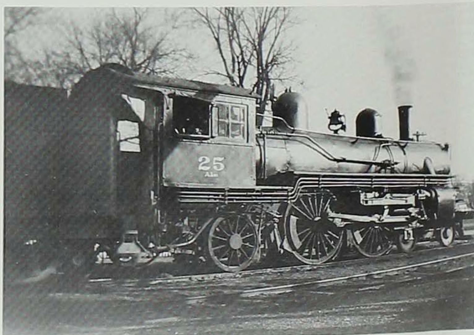
The two-car passenger train that arrived at Spirit Lake daily was often pulled by Engine No. 25, one of the small Atlantic-class locomotives.
