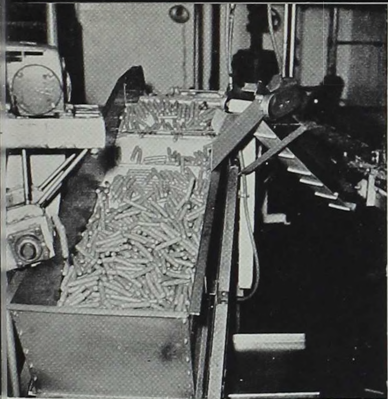
Automatic frankfurter loader in the Cedar Rapids plant collates and aligns 45,000 franks an hour, groups them into the correct number of franks per package, and delivers them to the vacuum packaging machine.
