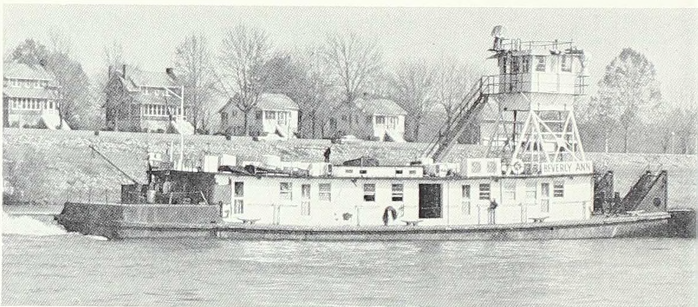
The Beverly Ann , originally the Pere Marquette , was a single propellor 900 hp boat with retractable pilothouse that was acquired by Alter Company in 1966. Sold to Pott Industries 1969 she was renamed the Port of Mobile .
