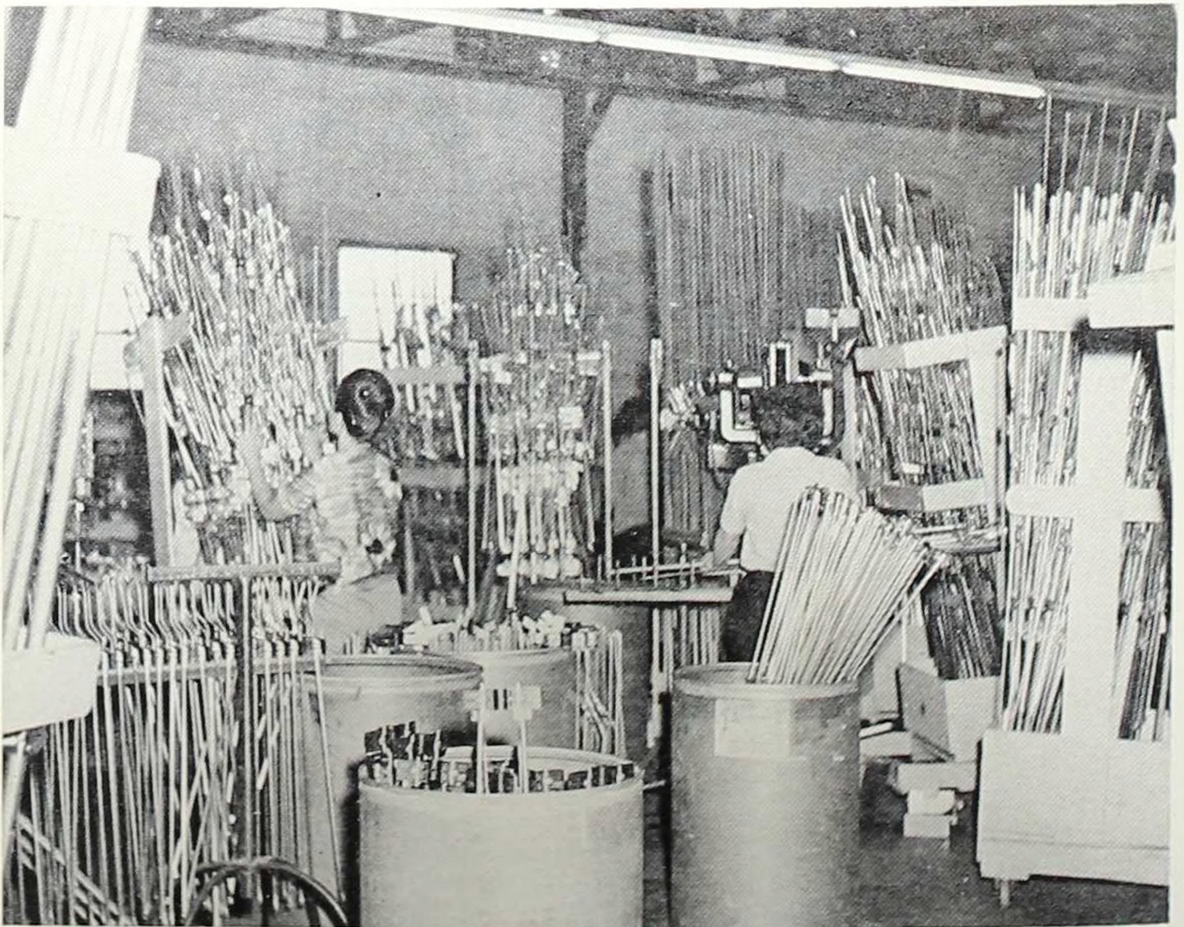
Storage area for aluminum antenna elements ready for delivery to the assembly line.
