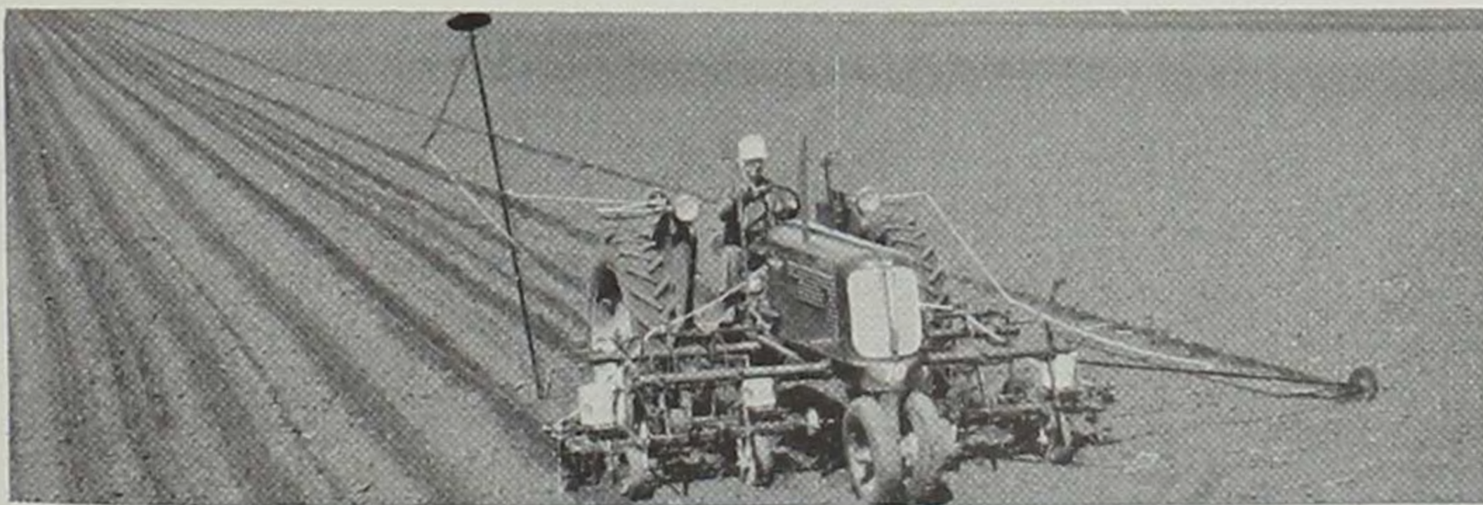
Four-row tractor planter with check rower.
