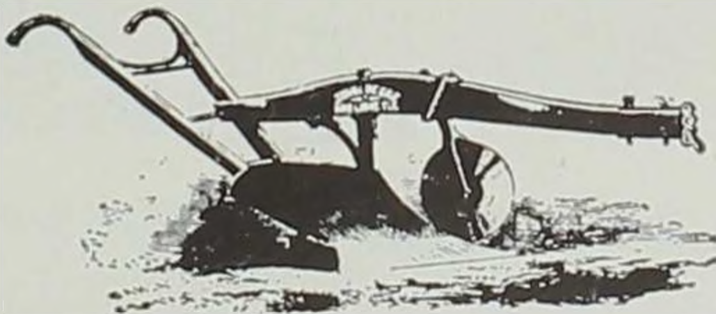
John Deere steel walking plow. From Ia. Agr. Soc. Rept. 1867.
