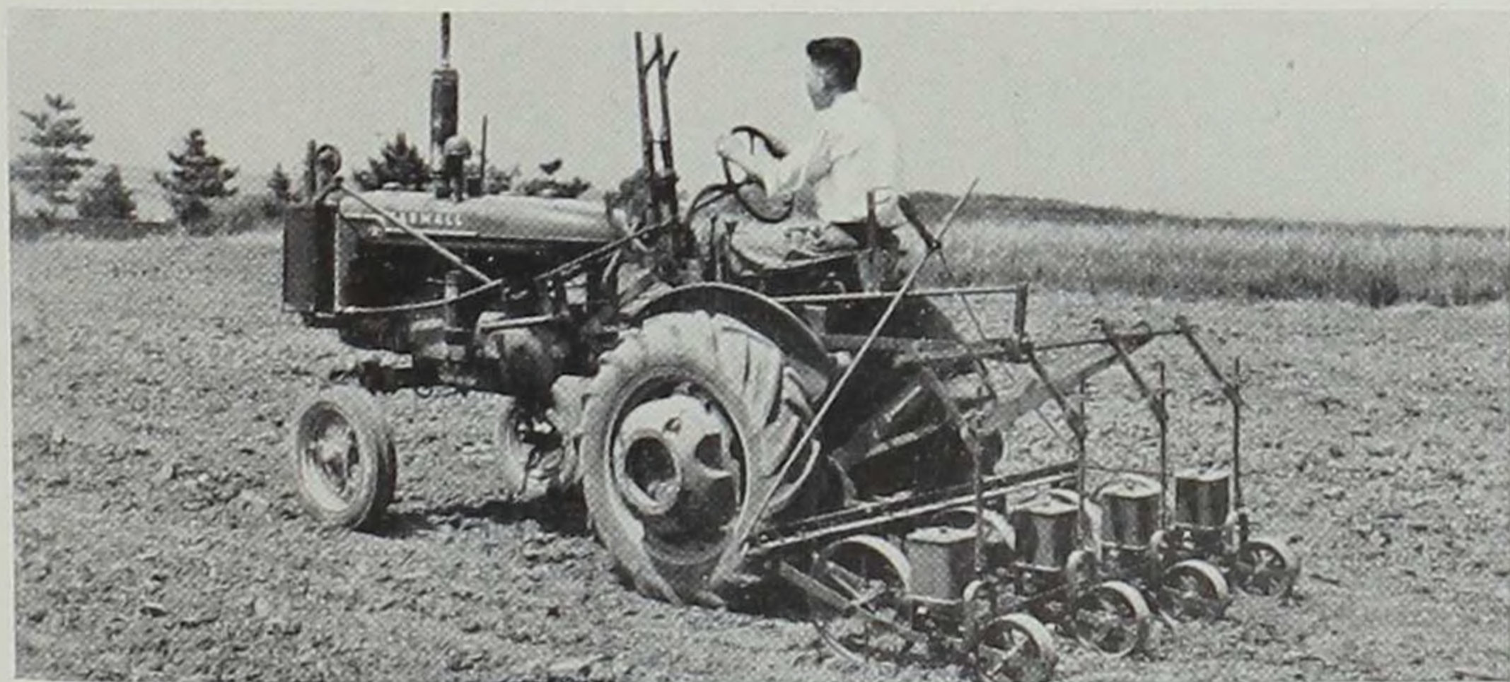
Direct connected four-row tractor garden drill.
