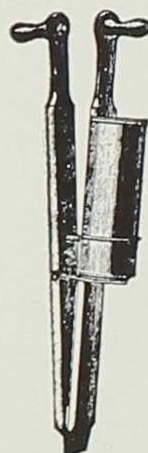
Hand planter. Opening handles releases seed.
