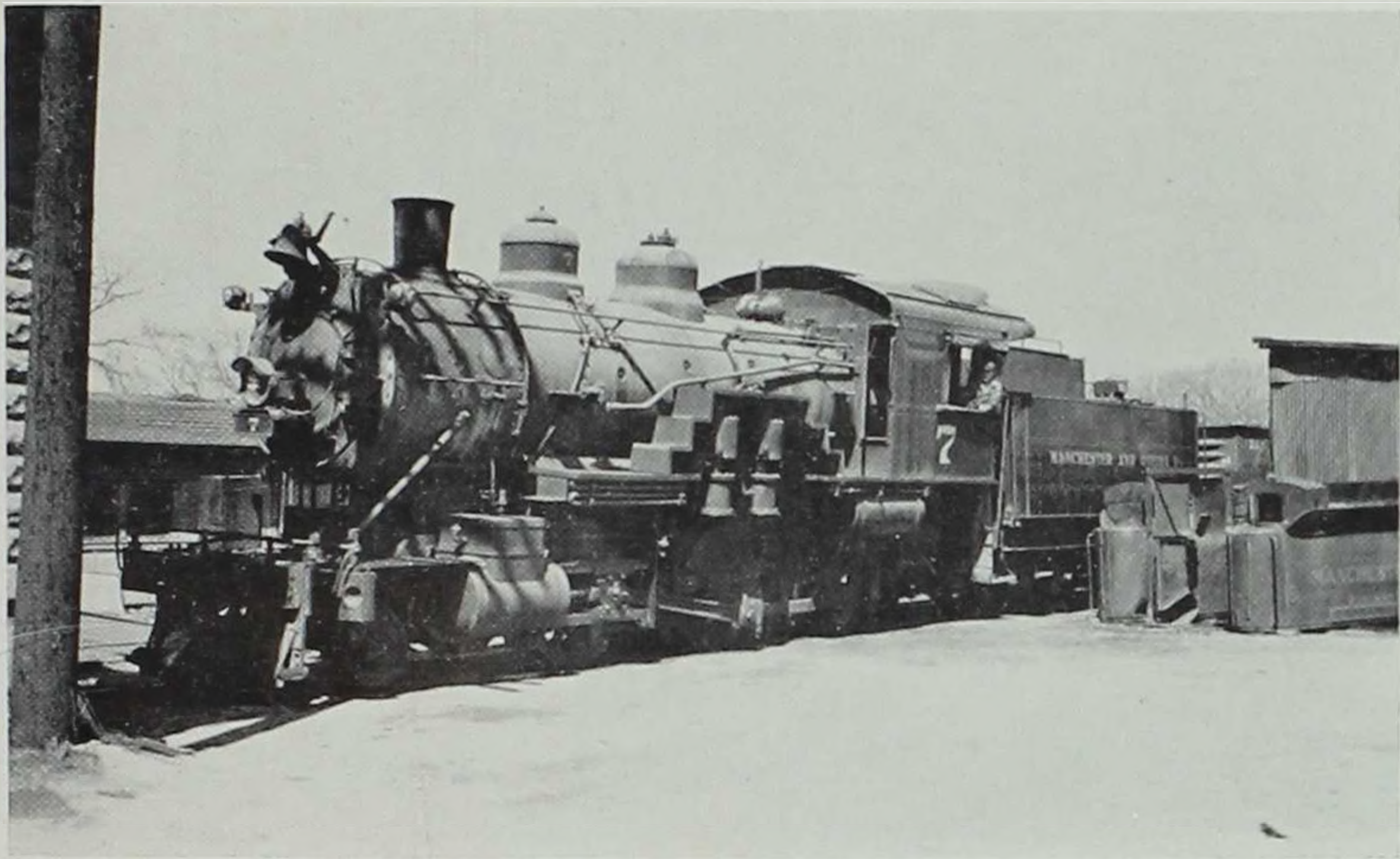
This Mogul, the last locomotive purchased by the M & O, was too heavy for the road's light rails. After constant derailments she was scrapped.
