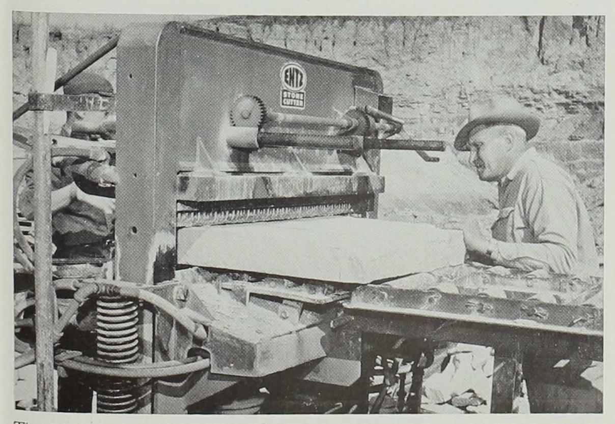
The conveyor carries the stone to this machine where it is cut into the desired size.
