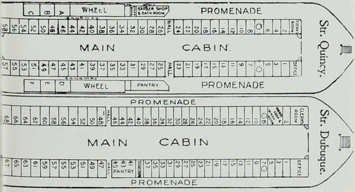
Cabin plans of a side-wheel and stern-wheel steamboat.
