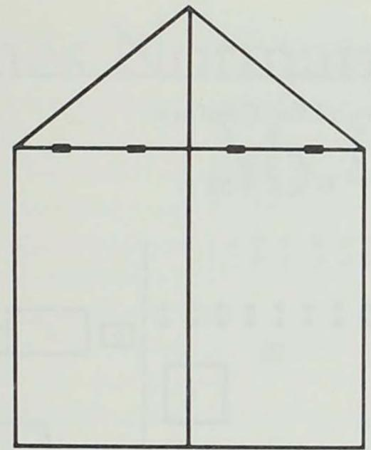
The hay door at the top of the south wall. The hinged top sections drop down, then the big doors open out. An inside platform makes opening and closing the doors easy. (design courtesy the author)
