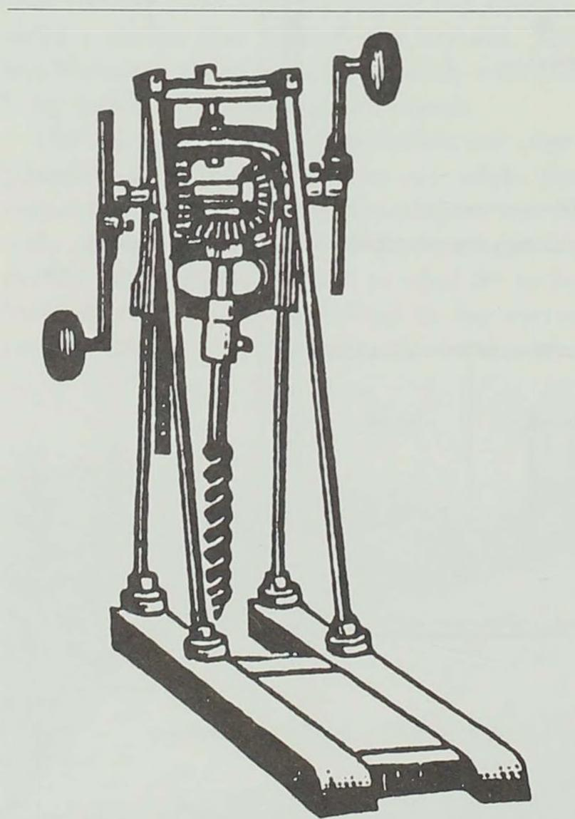
An adjustable drilling tool for peg holes and brace grooves.
