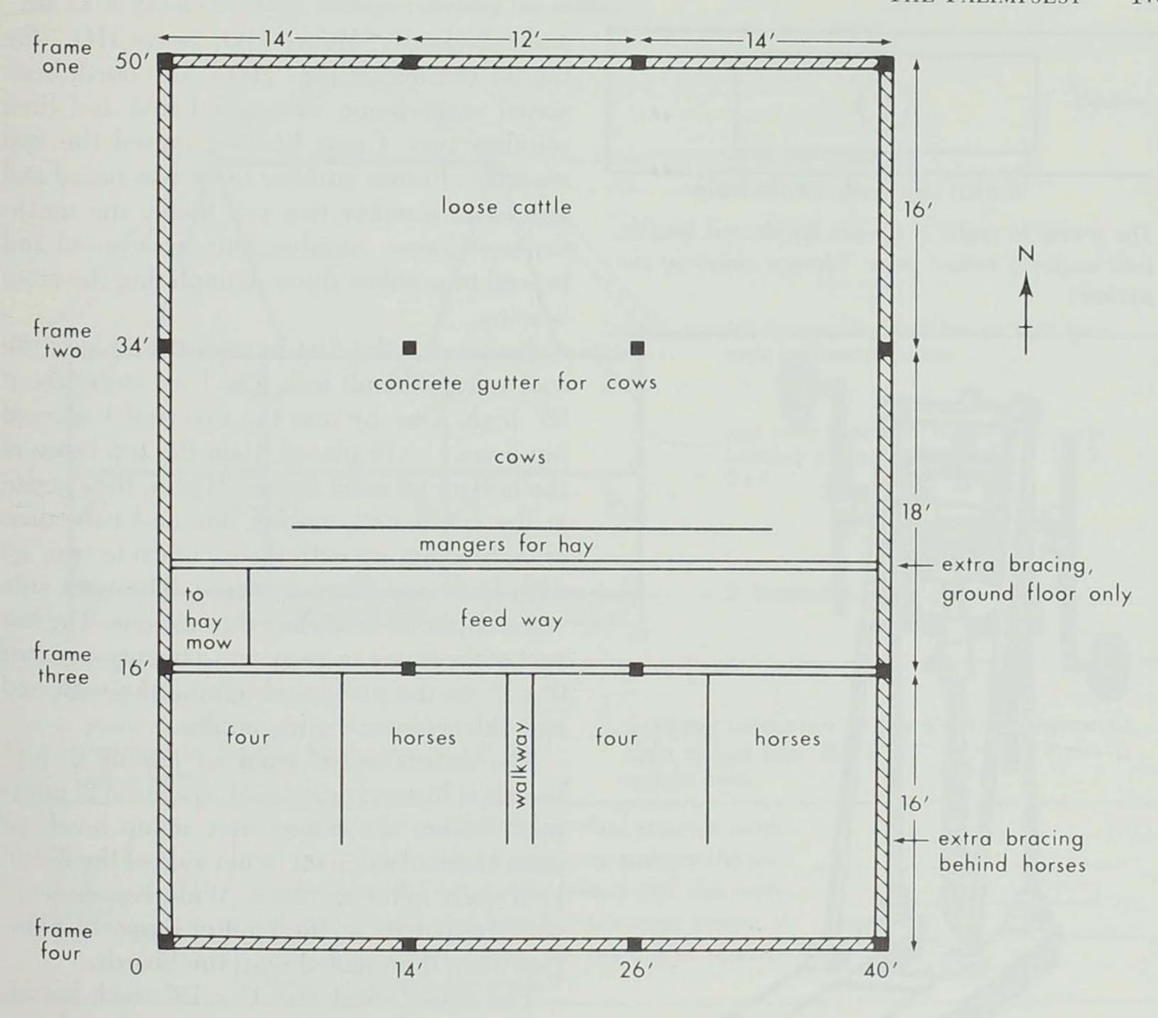
$\blacksquare$  = locations for main horizontal frame 6" × 6" posts (4 posts to each of four frames)
