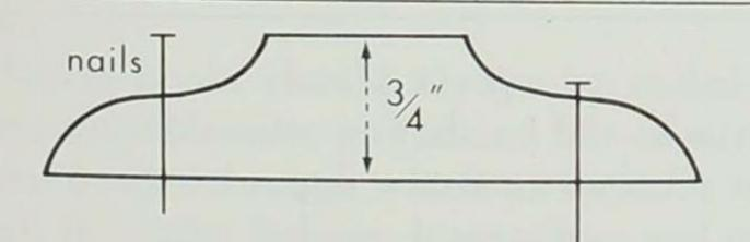
An end view of a batten to cover cracks between stock board siding. (design courtesy the author)
