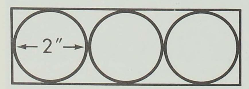
Circles were drilled with a 2" wood bit, then chiseled to make a rectangular notch to receive the braces. (design courtesy the author)
