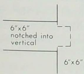
The drawings to the left (notched exterior vertical frame) and right (center join) suggest the way the horizontal frames were joined with the vertical main frame and how 6" x 6"s were joined to make horizontal beams of sufficient length. (design courtesy the author)
