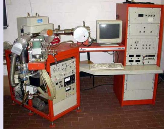
**Above:** Dan Pratt (1994) obtained the stable isotope data for this study using a Finnigan MAT 251 isotope ratio mass spectrometer similar to the one shown here. **Below:** schematic of a mass spectrometer. Once accelerated by the ion source, charged atoms of a particular element pass through the bending magnet where atoms of higher mass isotopes like <sup>13</sup>C are bent less than those lower mass isotopes like <sup>12</sup>C, thereby separating them to be counted in the collectors.
