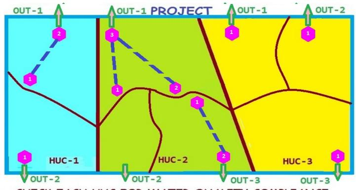
CHECK EACH HUC FOR WATER QUALITY COMPLIANCE CHECK EACH OUTFALL FOR CHANNEL & FLOOD PROTECTION DETERMINE RUNOFF AND POLLUTANT LOAD REDUCTION FOR EACH BMP.
