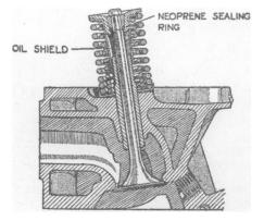
SECTION THROUGH A TYPICAL VALVE.
