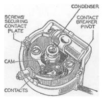
COMPONENTS OF CONTACT-BREAKER AS SEEN WITH COVER AND ROTOR REMOVED.
