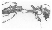
A SPECIAL TOOL-CUM-GAUGE CAN BE OBTAINED FOR " CAPPING " THE PLUGS.
