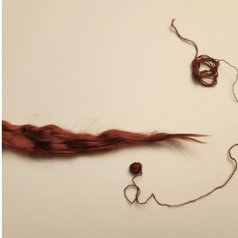
Figure 11. Unspun silk fiber next to a small ball of silk thread. Note the visible inconsistency in the thickness of the silk thread.
