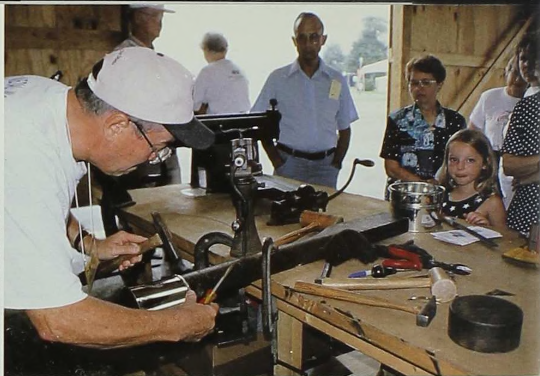
At the 1996 Festival of Iowa Folklife, Amana tinsmith Bill Metz uses traditional hand tools and presses to bend sheets of tin into pails, candle holders, and whistles. A retired metalworker, Metz follows traditional Amana forms.
