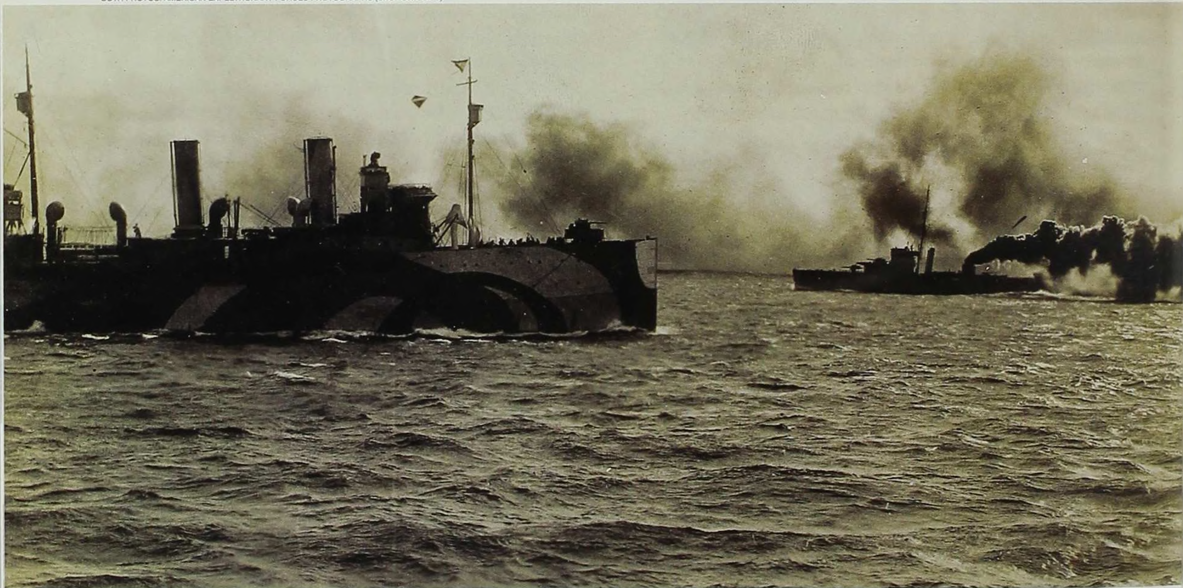
A splendid example of dazzle camouflage churns through the North Sea in September 1918. In this official U.S. Expeditionary Forces photograph, the H.M.S. Vampire circles the U.S.S. Shawmut with a smoke screen.
