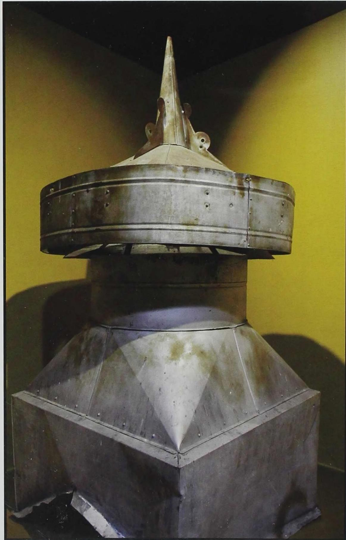
Designed to circulate air and dispel odors in a barn, ventilators like this one were commonly installed on barn roofs. This galvanized-steel Tip Top Ventilator was made in Des Moines by the Anderson Manufacturing Company and was used on a barn on the Van Pilsum farm near Prairie City about 1920.
