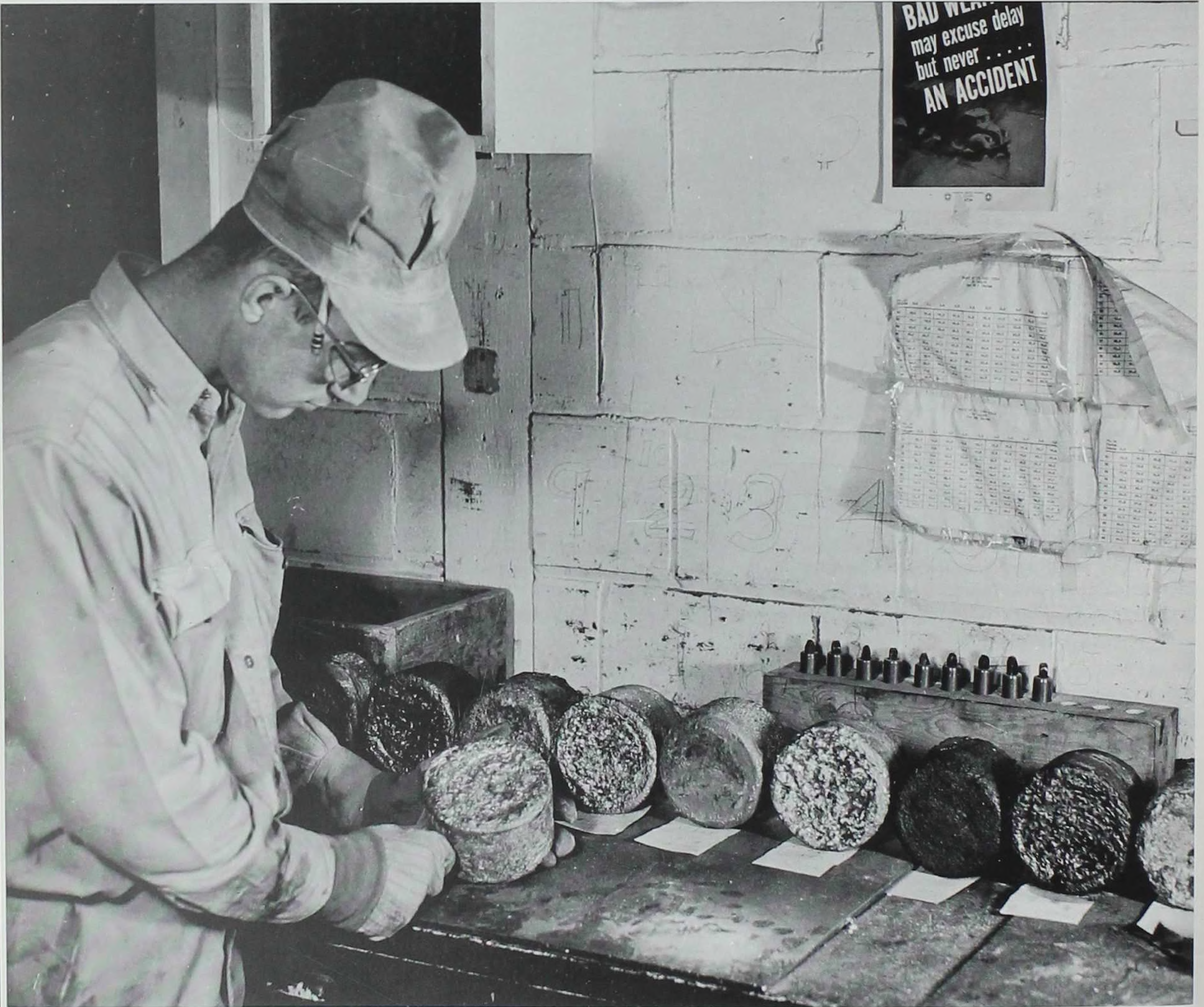
The uranium reduction process at the Ames Project yielded "biscuits" that could be cast into ingots.
