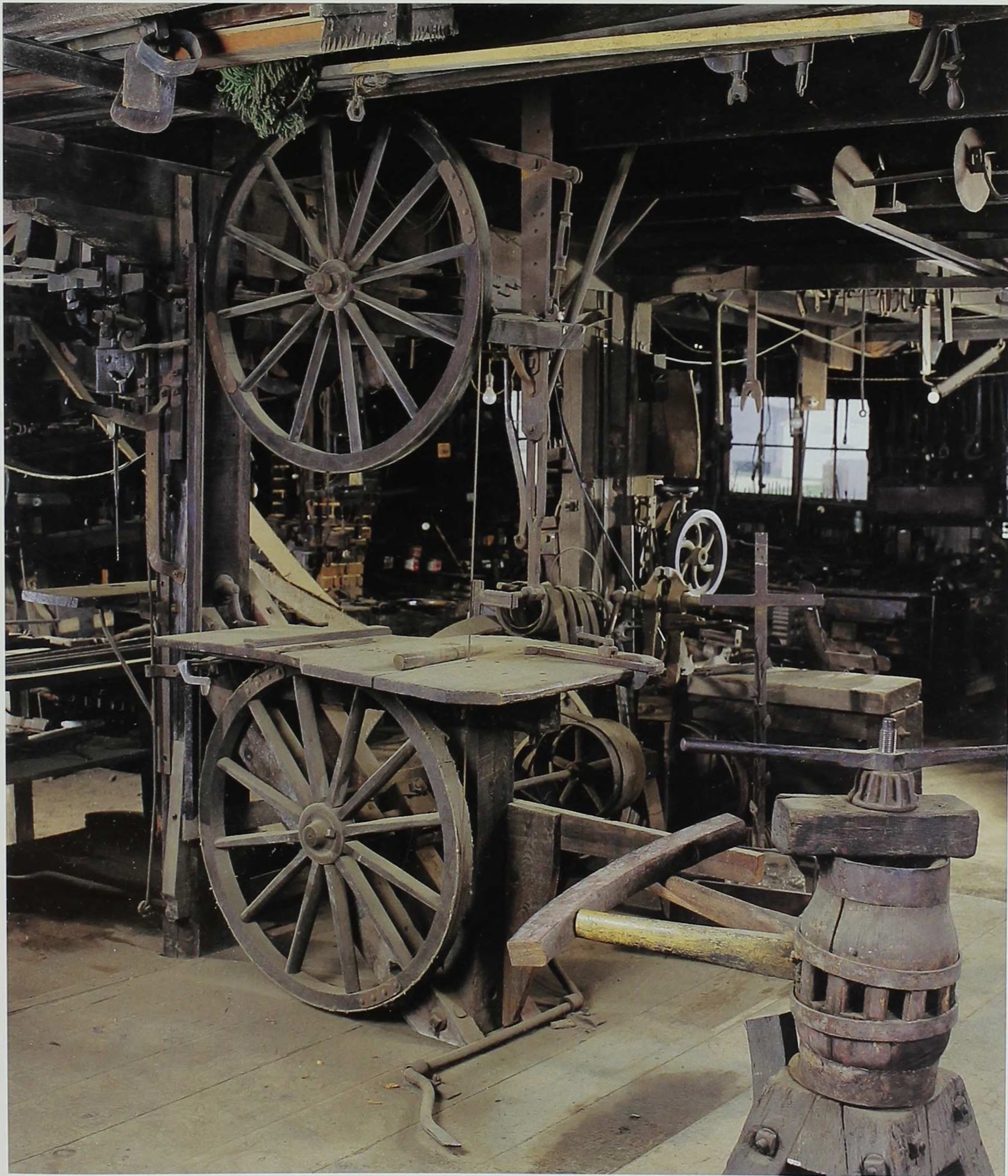
A portion of the shop was used for wagon repair and general woodworking, with a wide variety of hand tools nearby—braces and bits, hand saws and draw knives, planes and spoke shaves, chisels and gouges. The band saw, built into the rafters and floor, was fashioned from two custom-made wooden wheels. It could be treadled for small jobs, or line-shaft driven.
