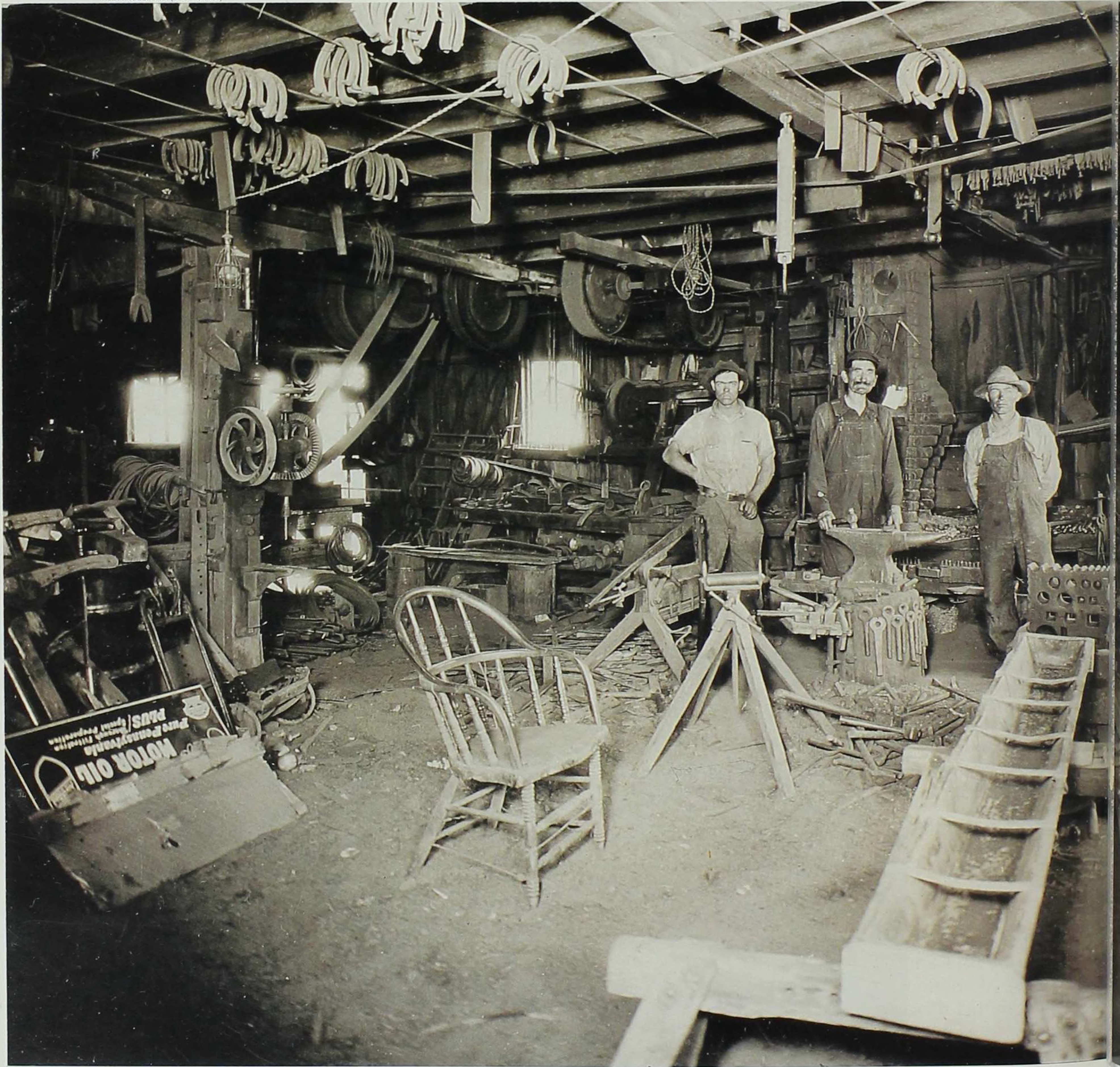
M atthew Edel is flanked by his son Louis and a local farmer, John Stalzer (on right), in this early 1930s photo of Edel's blacksmith shop in Haverhill, Iowa. In the front half of the shop, Edel did general forging and horseshoeing. General wood-working, wagon work, and manufacturing of tools were done in the rear half. A space under the stairway was used for plow grinding, and the half-story attic was used for storing wagon parts and other inventory. Of Edel's eight children, Louis was most involved in his father's shop.
