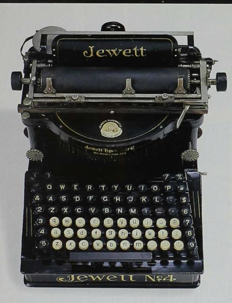
Double-keyboard typewriters like this one had separate keys for upper-case and lower-case letters. Patented by George A. Jewett, this model was first manufactured in Des Moines in 1892. Double keyboards, however, did not become the industry standard; instead, adding a shift key allowed for both upper- and lower-case letters. The Jewett Typewriter Company closed in 1910.
