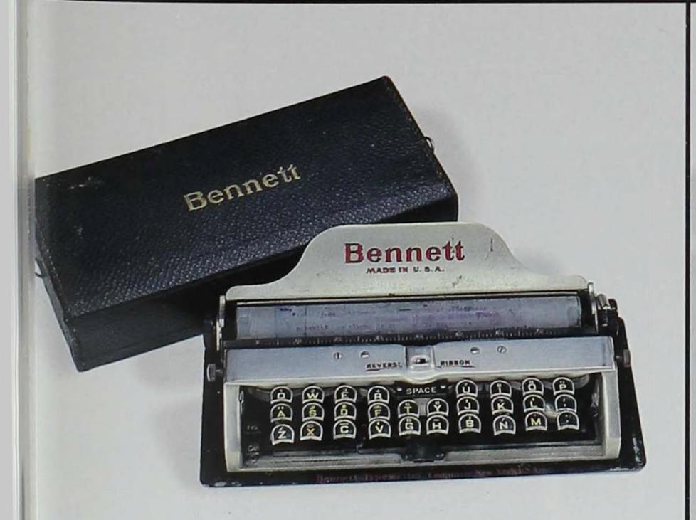
Because many early typewriters were large and heavy, some inventors worked to produce lightweight models. Charles Bennett introduced this typewriter in 1910. Tucked into its 11"x5" case and often made of aluminum, the Bennett weighed only a few pounds and could easily be carried in a briefcase or satchel.
