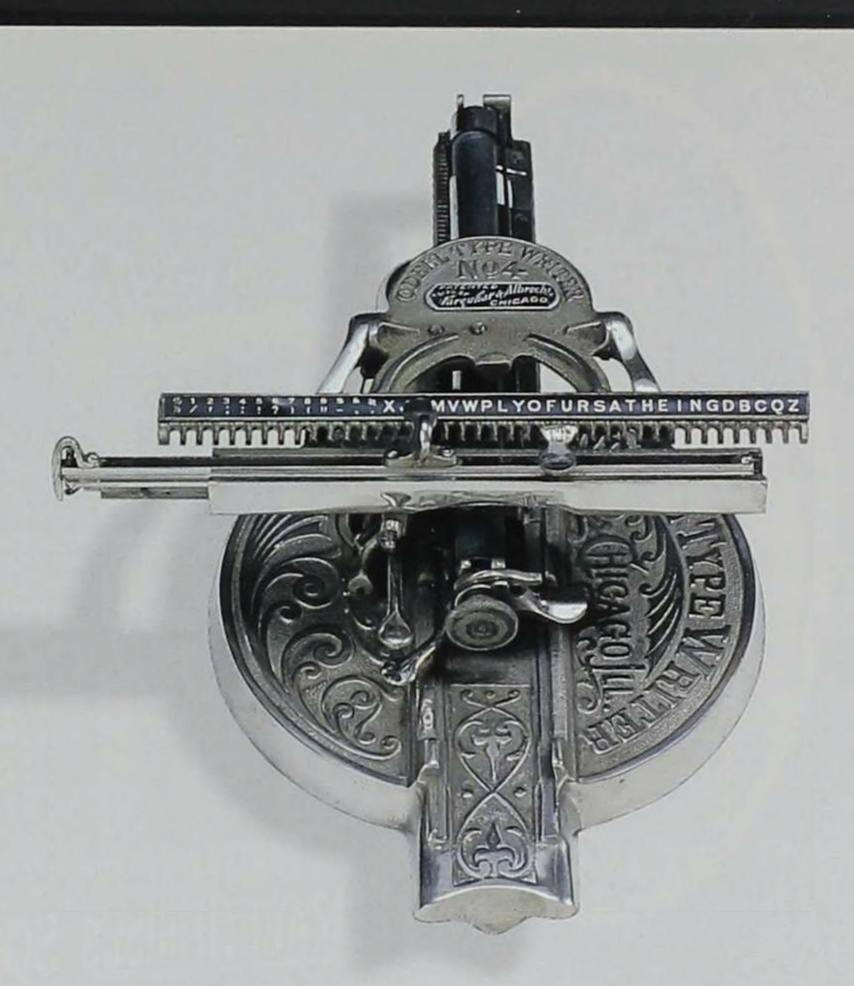
Index typewriters, like this Odell Model #4, operated by moving the linear type slide over the desired letter and pressing it to print. Levi Judson Odell of Chicago was granted the patent design in 1887; this machine appeared in 1904. Despite its low price, it was slow and soon vanished from the marketplace.
