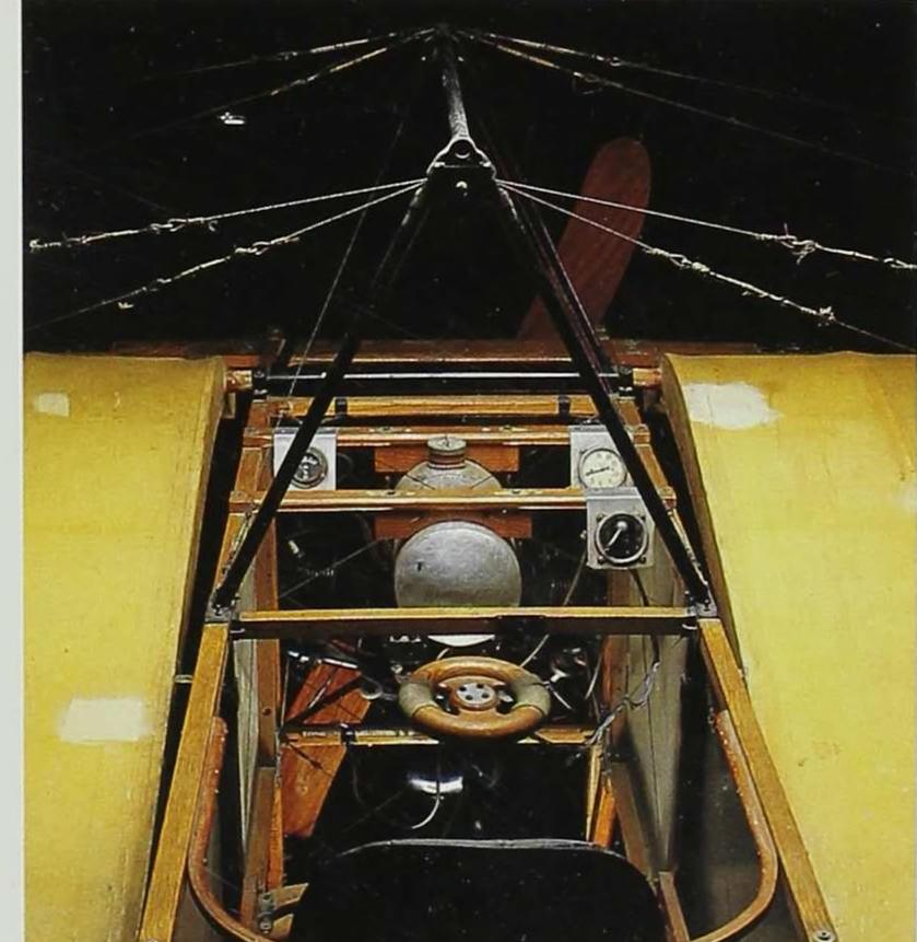
Left: Looking down into the pilot's seat of the Bleriot XI. Right: With no windshield, nothing broke the air flow on the Bleriot XI-except the pilot. Far right: To even out the stress on the plane, the pilot or mechanic tightened various metal turnbuckles on the wires; some are visible here on the tail.
