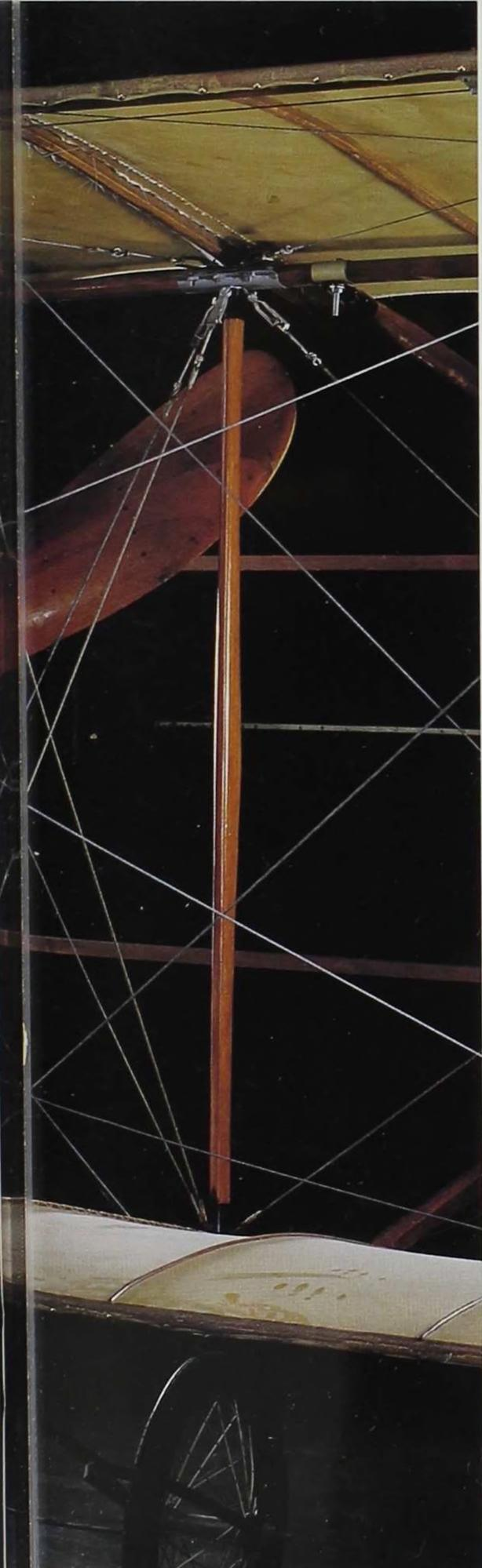
orking from plans in an aviation magazine, Ben and Arthur Klein built this Curtiss pusher (left) in their parents' barn near Treynor, Iowa, in 1911. They shaped the wood, formed steel brackets, strung wires, stretched fabric over the wings, and installed a \$500 engine. With Ben as ground crew, Arthur often flew the plane over the family farm.
