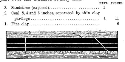
Figure 6. Clay seams in Topping Mine, south of Linden.
