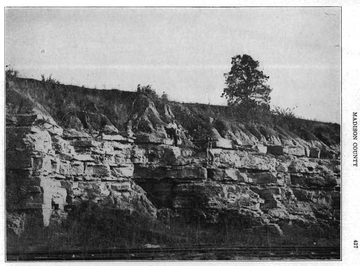
PLATE XXXV-Iowa Portland Cement Company quarry, Earlham, Madison county, showing the principal limestone beds with their characteristic clay partings.
