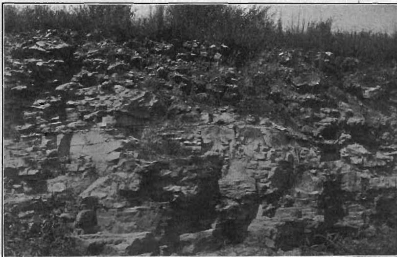
FIG. 64—Quarry in northern Lincoln township, Worth county, showing excellent material for road and concrete work.
