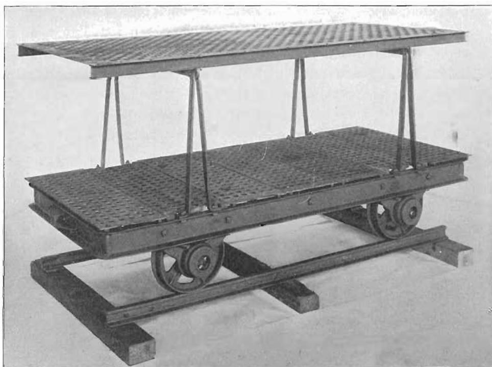
FIG. 25. Double deck steel car.
