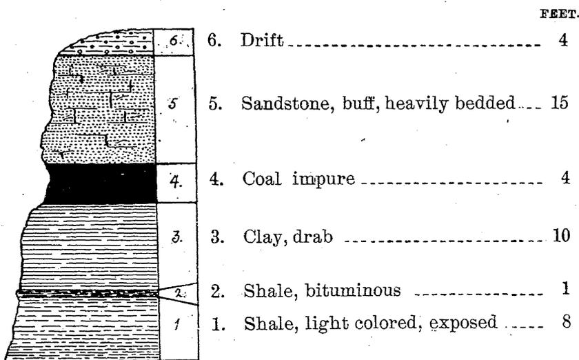
FIG. 51. Railroad cutting near east county line, below Runnells.
