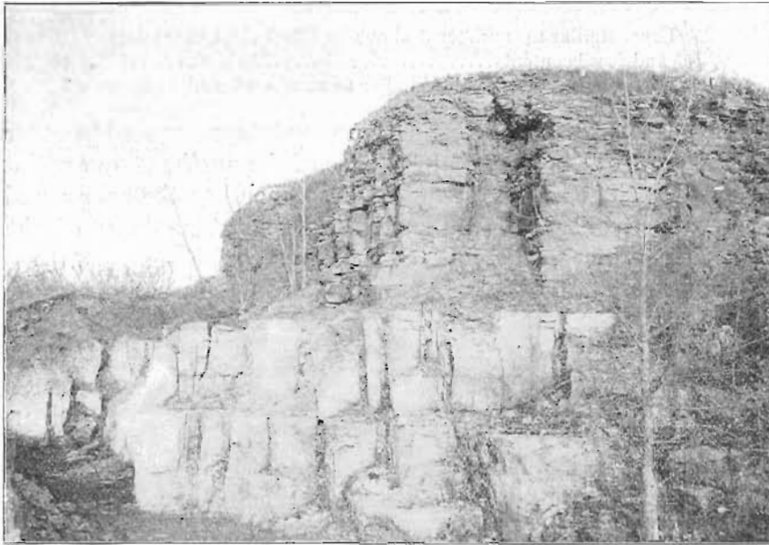
FIG. 29.—View in the Stevens' quarry in section 8, Indian Village township. The thin layers at the very top are limestone. The sand and impure limestone layers between contain numerous nodules of chert.
