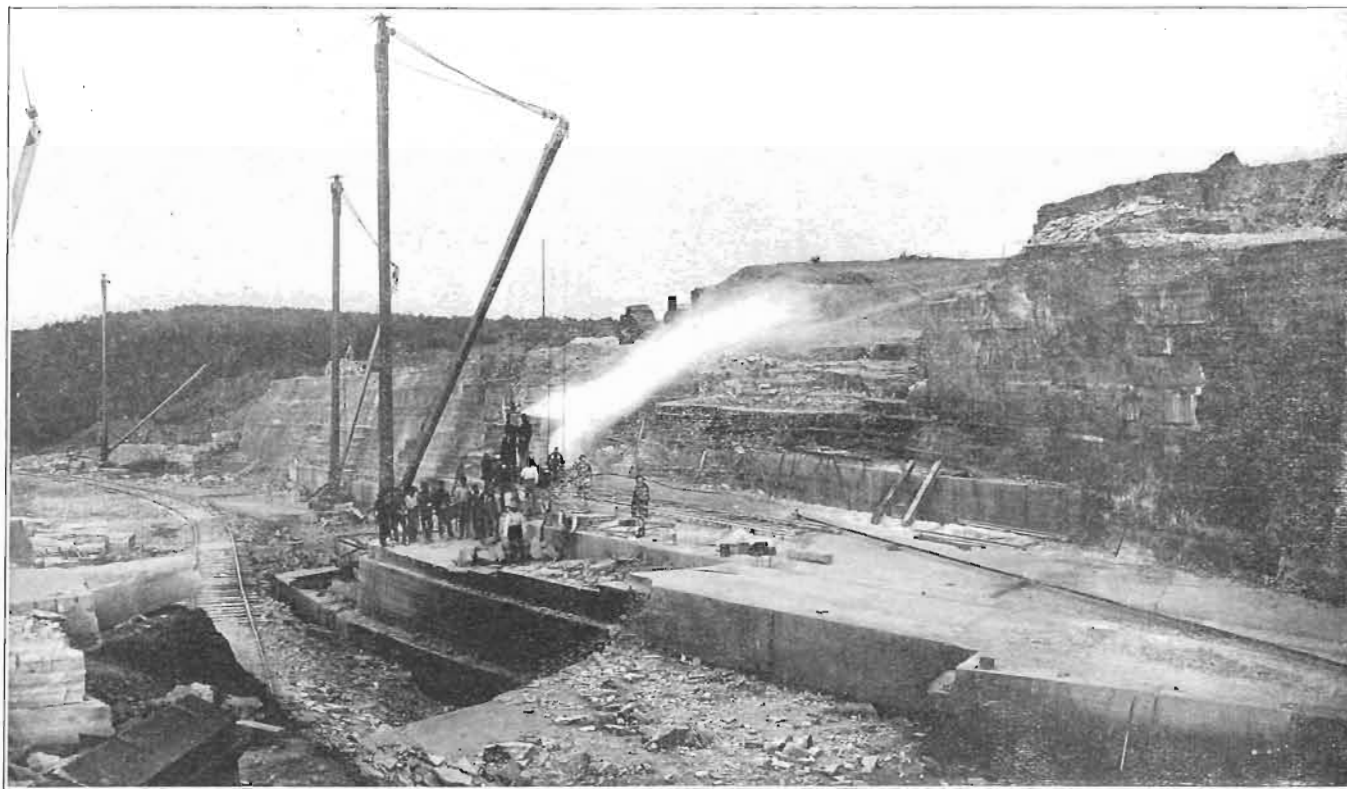
PLATE XLI—Champion quarry showing track and derrick arrangements and channeler. Stone City, Jones county, Iowa.
