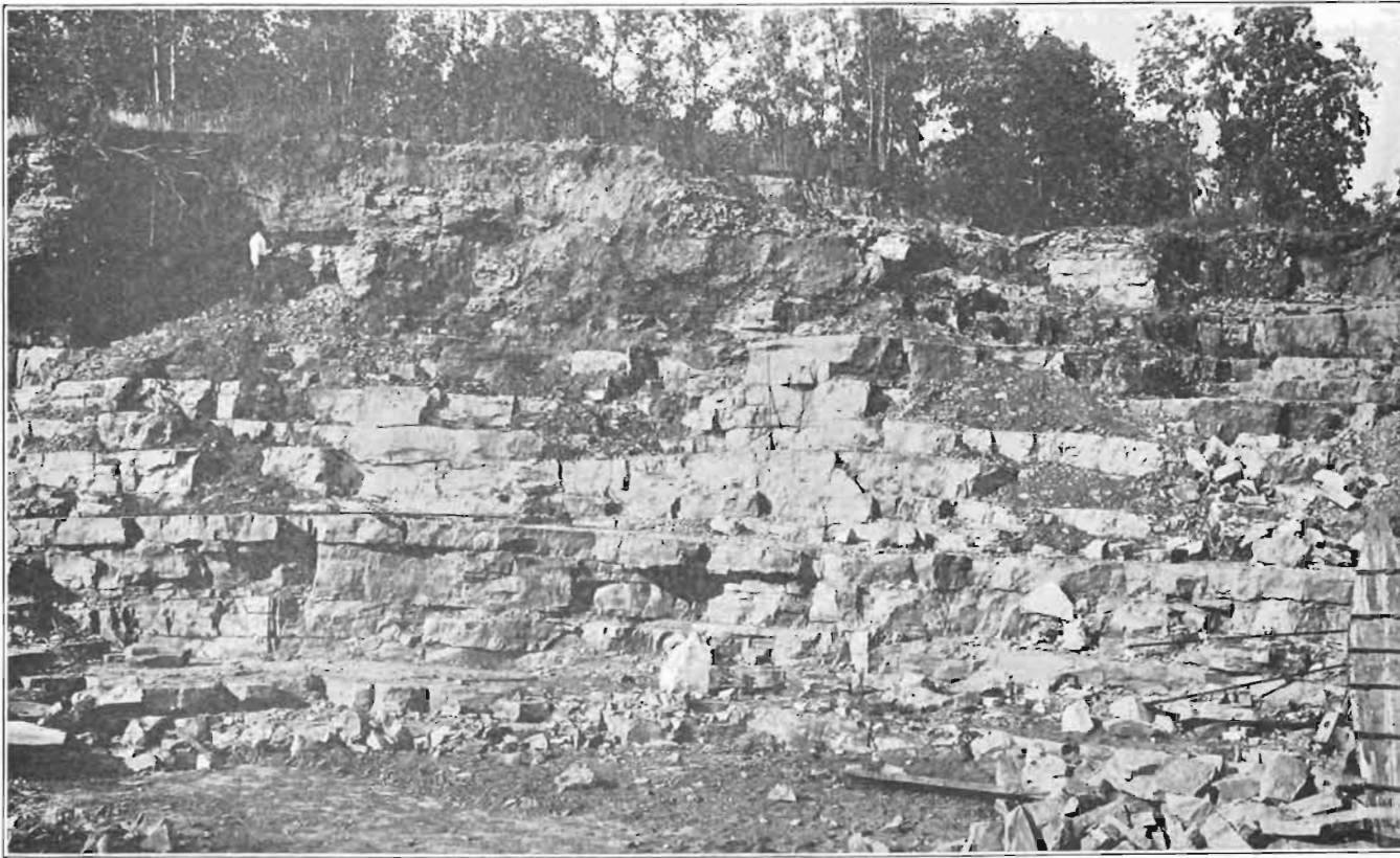
PLATE XLVI—Kuppinger quarry, Mason City, Cerro Gordo county, Iowa, showing the dolomite below, compact white limestone in the middle and the Stromatopora near the top of the section; an average section for the district.
