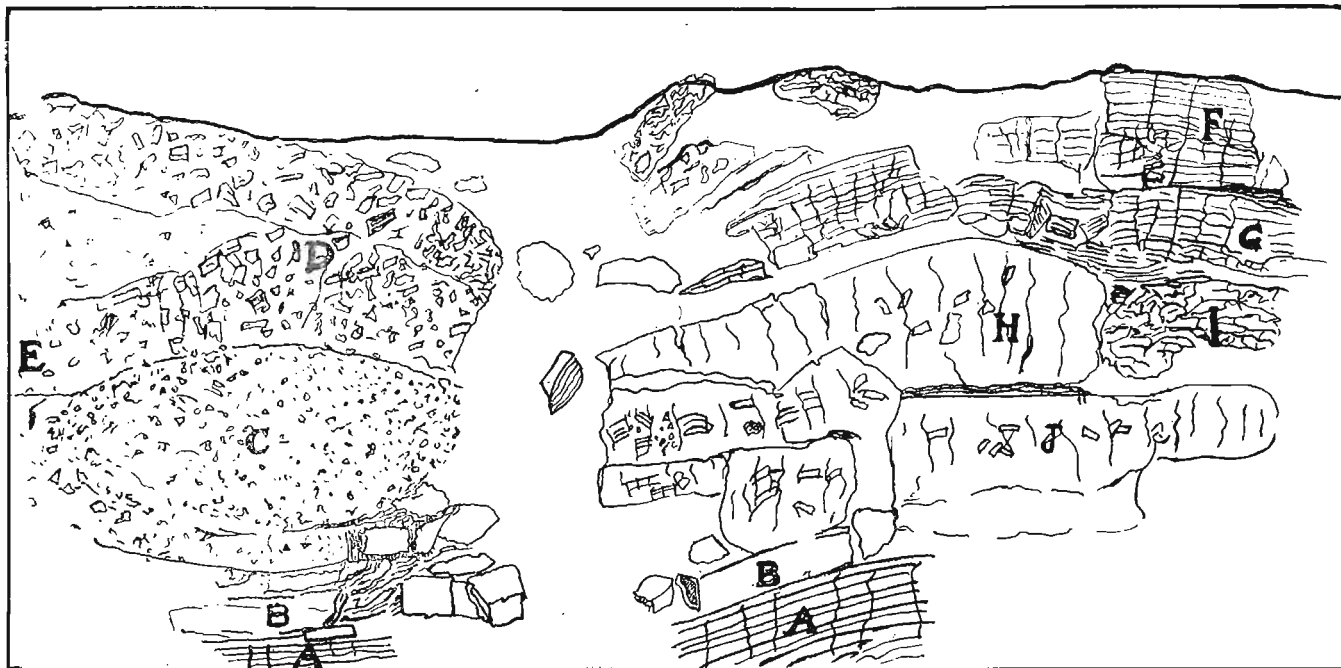
Section in City quarry, West Union, Fayette county. Outlines drawn from a photograph. A, Laminated Otis limestone, No. 2 of quarry section. B, Otis limestone, No. 3. C, Lens of broken Otis calcilitite continuation of H—J. D, Rubble of Otis breccia, many fragments of which are three to four inches in diameter. E, Rubble breccia of large Independence matrix with Otis fragments. F, Crackled laminated Otis calcilitite, in places a mosaic breccia. G as F, but somewhat more brecciated, faulted, and laminae bent in places and rotated. H, Massive, finely crackled and some fragments displaced. I, Mosaic breccia. J, Ruptures chiefly vertical, mosaic-crackle breccia.
