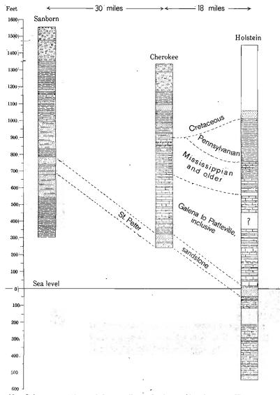
FIG. 63. Columnar sections of deep wells at Sanborn. Cherokee and Holstein. (Norton, Iowa Geological Survey, volume XXI, page 1006.)
