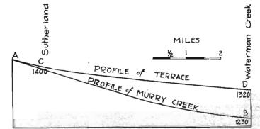
FIG. 57. Profiles along Murry creek valley from Sutherland to its mouth, showing, A-B, the gradient of the creek, and, C-D, the gradient of the terrace.
