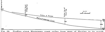
10. 56. Profiles along Waterman creek valley from west of Hartley to its mouth, showing, A-B, the gradient of the stream, and, C-D, the gradient of the terrace.
