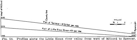
'IG. 54. Profiles along the Little Sloux river valley from west of Millord to Spencer, showing the gradient of the river and the gradient of the terrace. The distance is measured along the central line of the gravel-filled area. The fall of the river from west of Milford to Spencer, measured along its winding course, is two and two-thirds feet per mile.
