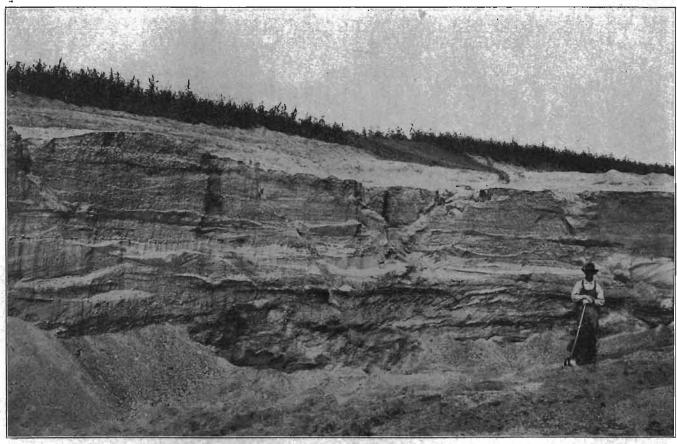
Lehatchka and Pattengill pit about half a mile north of Rock Rapids, Lyon county. The view shows cross-bedding and basin structure, variation in the coarseness of the material, and the thickness of the stripping. (Beyer, Iowa Geological Survey, volume XXIV, Plate XXXII, page 421.)
