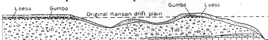
Fig. 5.—Diagram showing relations of super-Kansan "gumbo" and of loess to remnants of the original Kansan drift plain.
