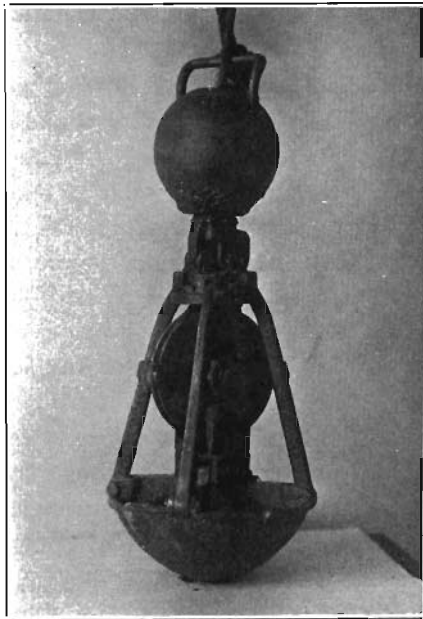
FIG. 17. — Orange-peel bucket, used with 12-inch casing.
