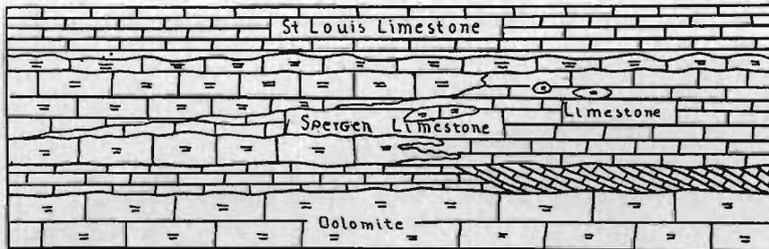
FIG. 35. Showing relations of dolomite to limestone at one point in quarry face, three-fourths mile south of Belfast, Iowa. Scale, one inch=twelve feet.
