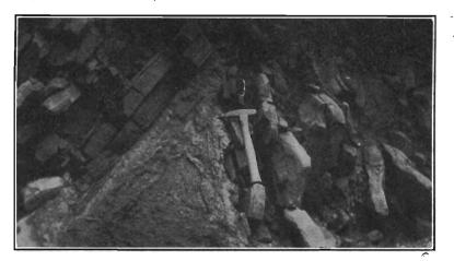
FIG. 70.—Small slump fold involving the Maquoketa shale and the overlying Edgewood beds. Southwest quarter, section 14, Prairie Spring township, Jackson county, Iowa.
