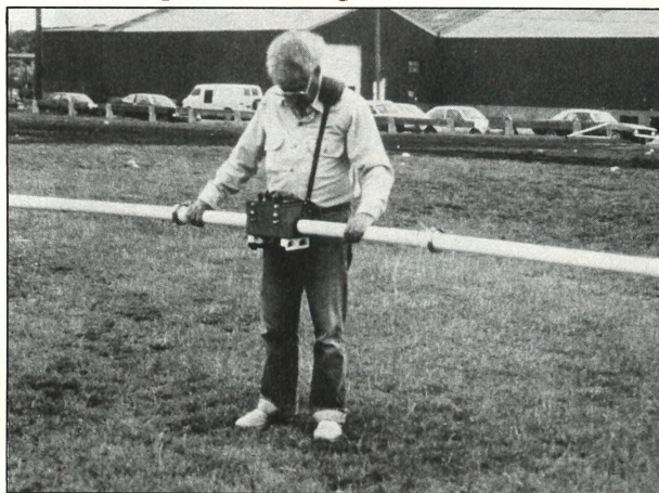
A man uses ground-penetrating radar to find disturbances in the soil. Radar waves are sent out from the poles into the ground.
