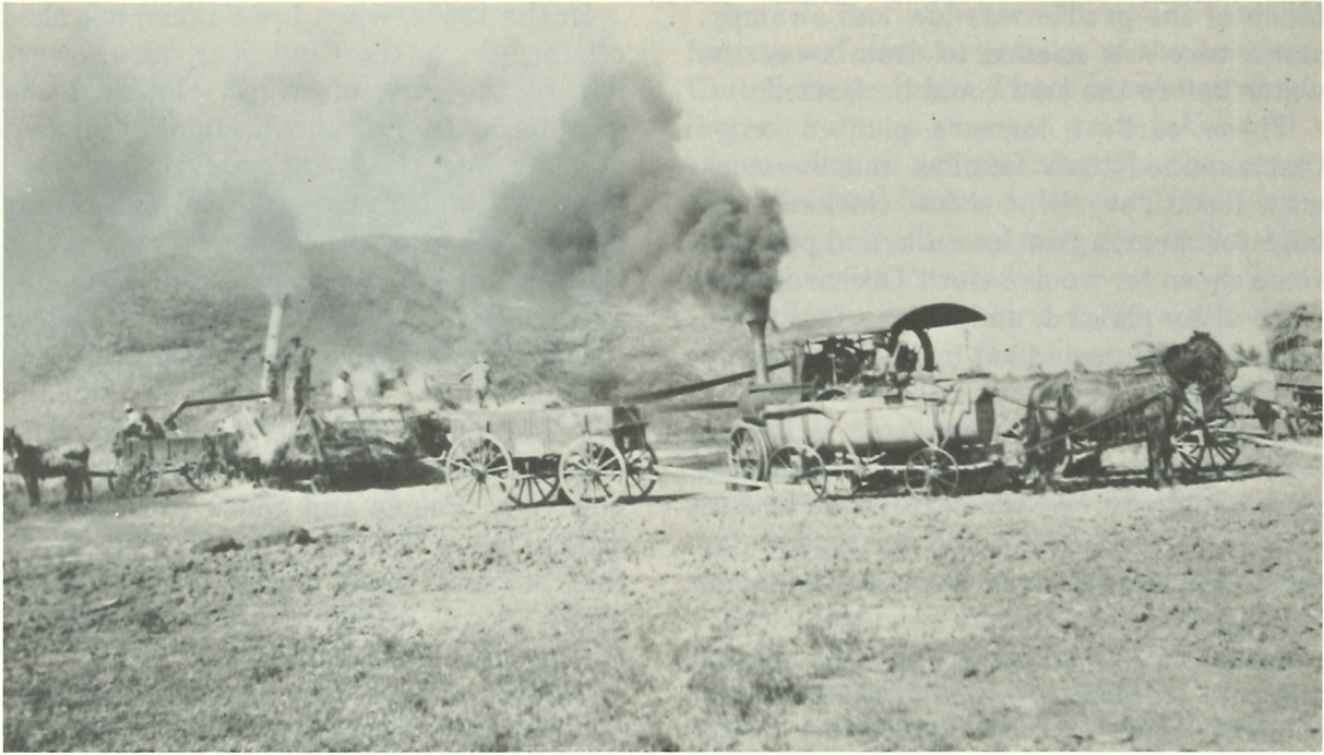
A steam engine belches black smoke as it powers the threshing machine.
