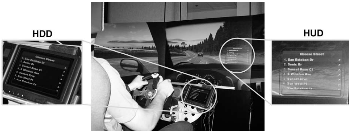
Figure 1. HDD (left) and HUD (right) variants of our prototype IVIS (shown together for illustrative purposes; only one at a time was used in the experiment)
