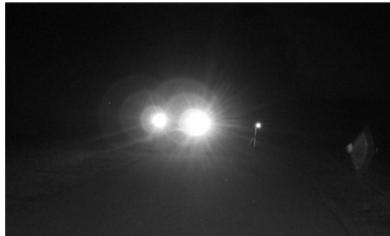
Figure 1. Position of the Landolt C stimulus in relation to the glare vehicle (both the glare vehicle and the participant vehicle are using high beams; the camera flash was not used)
