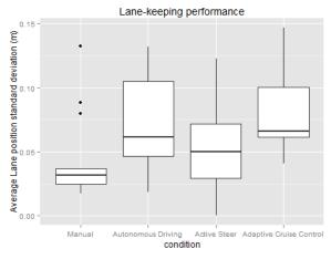
Figure 6. Lane-keeping performance measured by std. dev. of position from center of lane. [Box from the 25<sup>th</sup> to 75<sup>th</sup> percentile, bold line shows mean, whiskers extend to furthest point within 1.5\*interquartile range from the box, data points beyond that (outliers) are marked with a dotl
