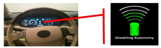
Figure 3. Steering wheel with mode switch button marked in green. The same button enables or disables the automated driving features, and the mode switch is only enabled in specific transition zones
