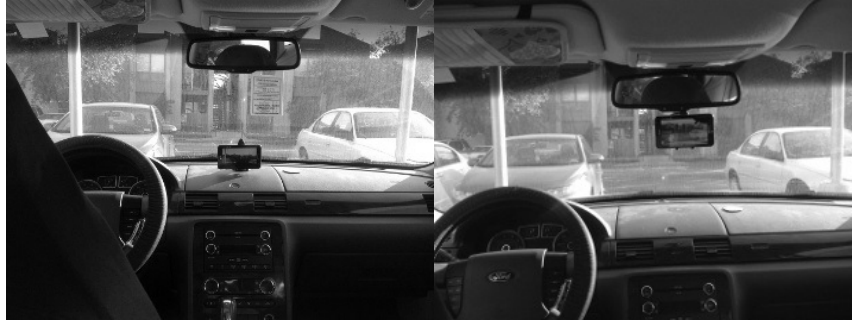
(a). A smartphone mounted on the dashboard (b). A smartphone mounted on the windshield Figure 1. The system setup of vehicle detections using a smartphone
