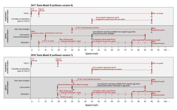
Figure 1. Available features on a Tesla Model S (software versions 7 & 8) that assist the driver in sustained DDT subtasks. Features are grouped based on their assisted vehicle motion control directionality (in lighter grey box – longitudinal; in darker grey box – lateral). Each line shows an individual system's functional speed range. Additional conditionality is noted above each line. TACC = "Traffic-Aware Cruise Control"
