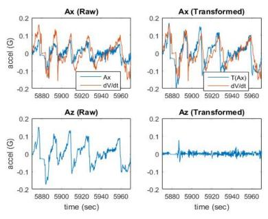
Figure 1. Transformation to normalize acceleration signals
