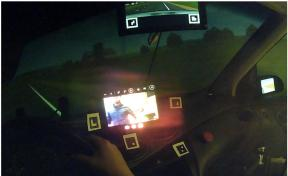
Figure 1. Participants operated a simulated vehicle and wore a HoloLens augmented reality (AR) device (left). HoloLens projected an AR Skype window for communication with a remote conversant (right).
