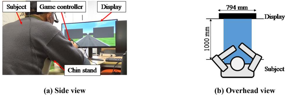
Figure 3. Test situation of SART with optical flow
