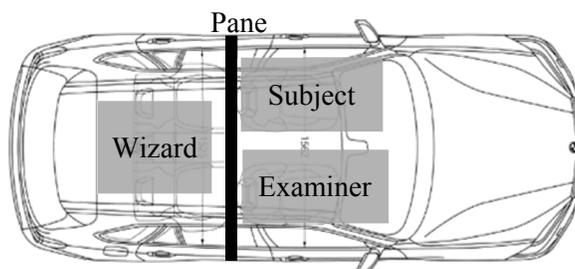
**Figure 2. Concept of Wizard-of-Oz vehicle for CAD (Gold, Meyer & Fischer, 2018)**
