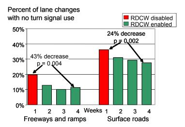
Figure 2. Increase in use of turn signals during lane changes
