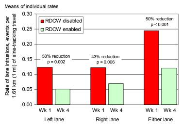
Figure 3. Reduction in the rate of events in which vehicle edge comes within 0.1m of lane edge
